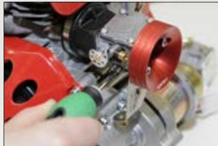
then you should carefully screw in the High Speed screw one tenth of a turn. **WARNING!** Do not overdo it and screw in the High Speed screw too much, because then the engine will not receive enough fuel and as a result not enough oil, which can lead to piston and cylinder damage. The High Speed screw should always remain opened at least a 0,75 turn.
