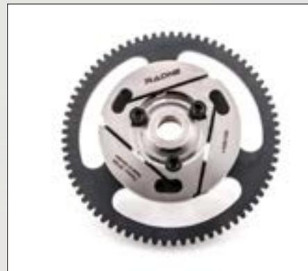
other words it is not permitted to change the clutch weights or the clutch springs in order to alter the number of rpm at which the slip clutch engages.
