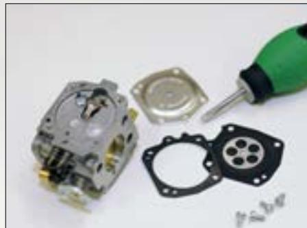
kets on the pump side will exhibit the same symptoms. If the opening or sealing pressure is not correct then you will have to change the spring and lever until it does appear to be correct.
