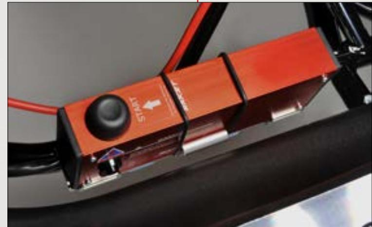
3. The start button and the charger plug can be found on the battery box. In the box there is also a 40 A fuse that prevents the battery from being destroyed if a short should occur outside of the battery box. The fuse may only be changed for an identical fuse that can be purchased as a spare part from a Raket reseller.
