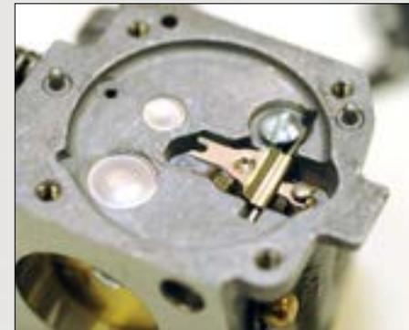
the engine. All gaskets should be OK. Ensure that the hose running from the crankcase to the carburettor is in place. Press carefully (we emphasise – CAREFULLY) down on the master diaphragm which you can reach through the small hole on the die-cut cover of the carburettor. When you press down on the diaphragm the inlet valve opens. Turn the engine around and check to see if there is any fuel coming from the tank.
